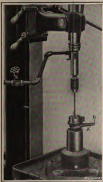
Fig. 17. Thread Cutting on a Drilling Machine with Stationary Self-opening Die.
